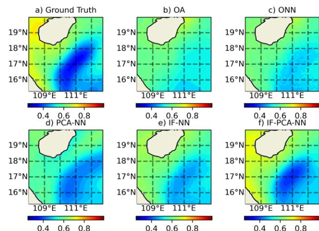
Fig. 8. The sea surface height (unit: m) for region A on March 26, 2020 where a) is the HYCOM original field, b-f) are the OA, ONN, PCA-NN, IF-NN, and IF-PCA-NN results, respectively.
