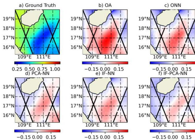
Fig. 9. Same as Fig. 8 but b-f) are the deviations of the OA, ONN, PCA-NN, IF-NN, and IF-PCA-NN reconstructions from the ground truth. The black lines mark the trajectory of Jason-2.
